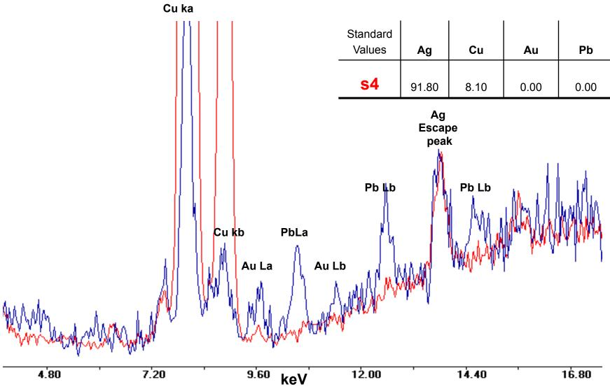
This is an overlay of standard **s4** (**red**) that contains no Au or Pb and the **tureen interior** (**blue**).. It is apparent that the tureen does contain traces of both Au and Pb. I would estimate both to be around 0.02 %.
