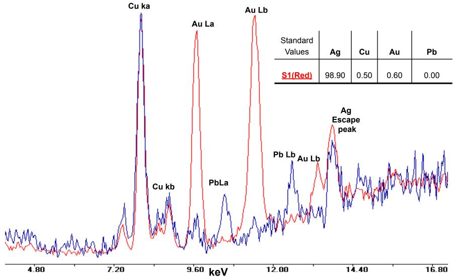
This is an overlay of a standard **s1(red)** that contains 0.60 % Au and no Pb, and the **tureen interior (blue)**. It is apparent that the tureen does contain traces of both Au and Pb. I would estimate both to be around 0.02 %. Also comparing the tureen to the standard shows that the Cu content is about 0.50 %
